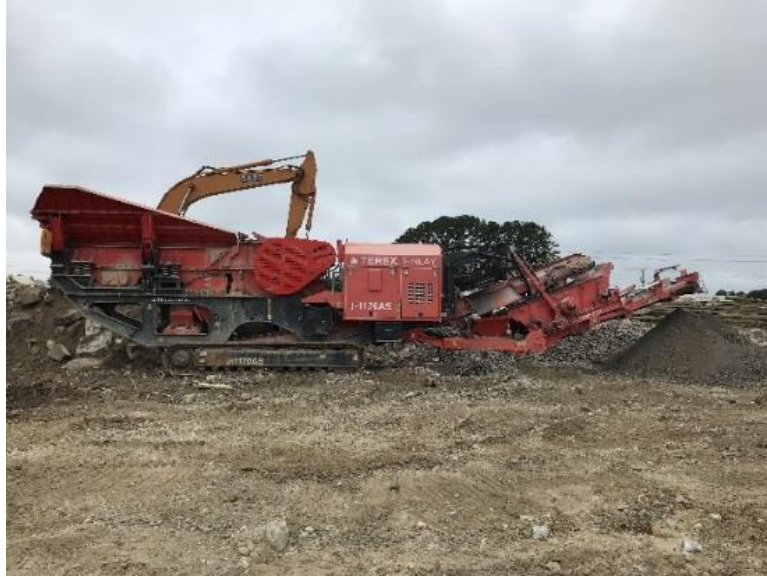
Figure 4.2.5 Terex Finlay J-1170 Compact Crusher Used for RCA Processing
