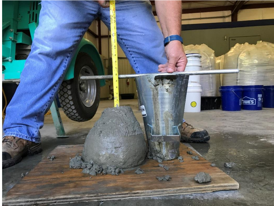
Figure 12.12.49 Slump Test of Fresh RCA Concrete
