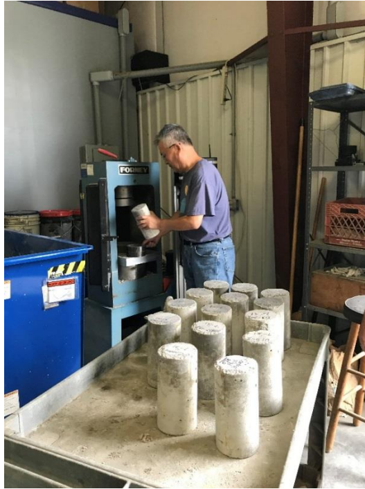
Figure 12.12.53 Compressive Strength Test
