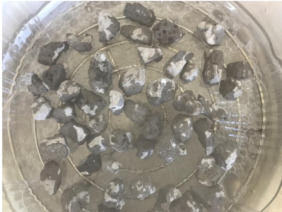
Figure 12.12.34 EAF Slag Underwent Pressure Cooker Test
