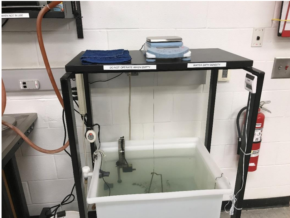
Figure 12.12.30 RCA Bulk Specific Gravity Testing
