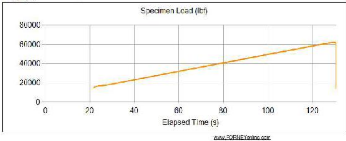
Figure 12.9.68 20%EAF Slag + 80%RCA Concrete 90-day Strength
