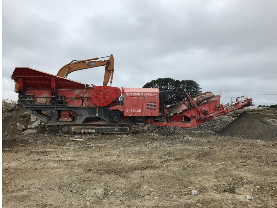
Figure 12.12.7 Terex Finlay 3-in-1 Crusher Used in the Process
