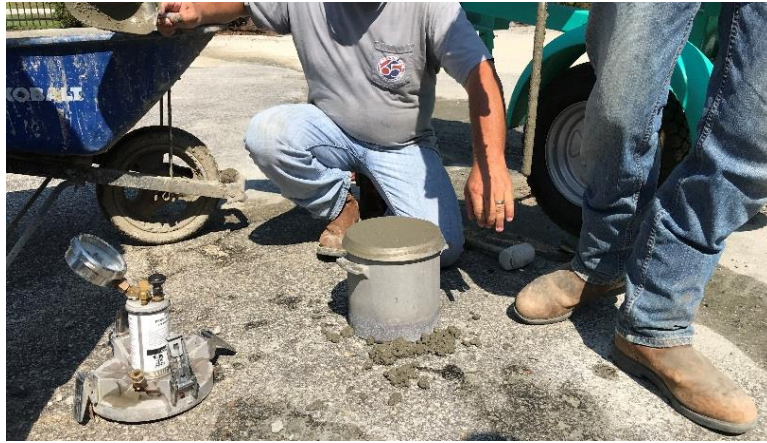
Figure 5.2.2 Unit Weight and Air Content Test of Fresh Concrete Containing RCA
