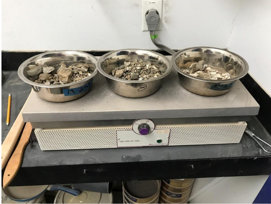
Figure 12.12.31 Absorption Test Before Mixing
