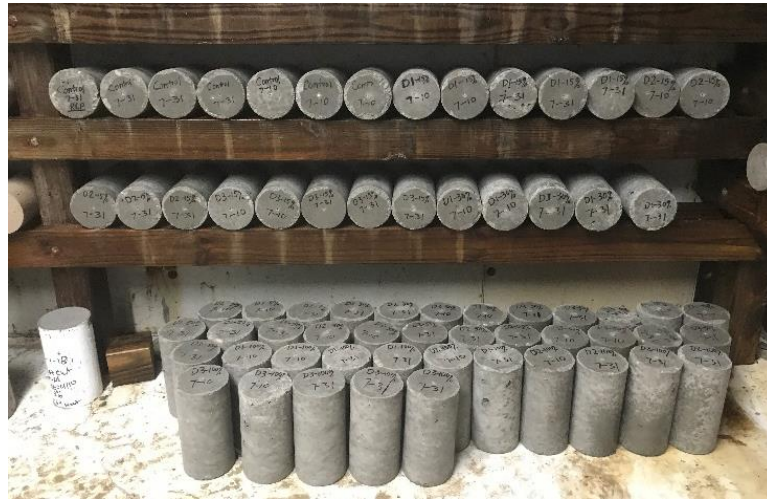
Figure 5.3.1 Concrete Cylinders in Curing Room
