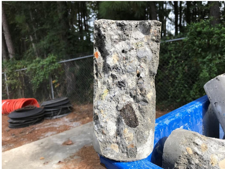
Figure 12.12.56 Broken Cylinder Containing RCA and EAF Slag
