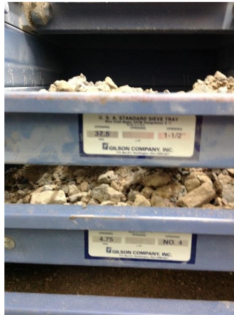
Figure 4.3.1 Screening to Obtain Particles Between #4 and 1.5 inch
