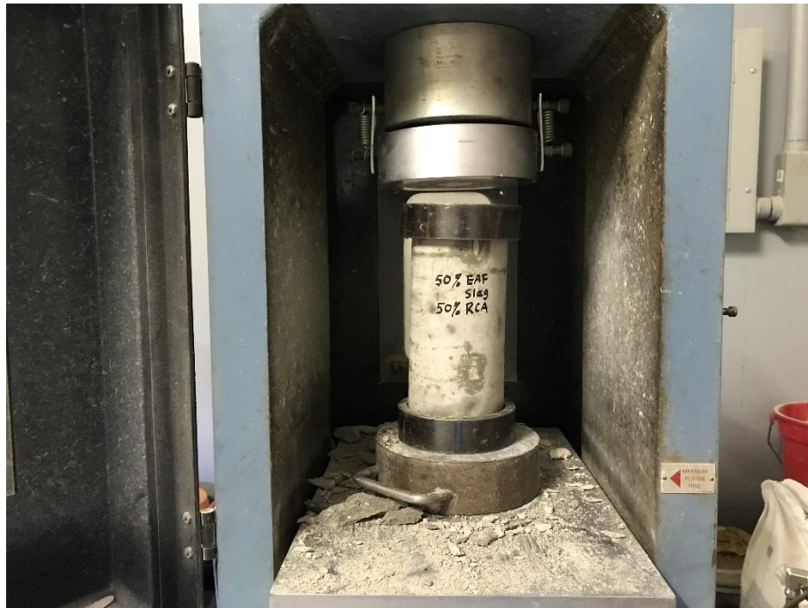
Figure 12.12.55 Breaking 28-day Concrete Containing RCA and EAF Slag
