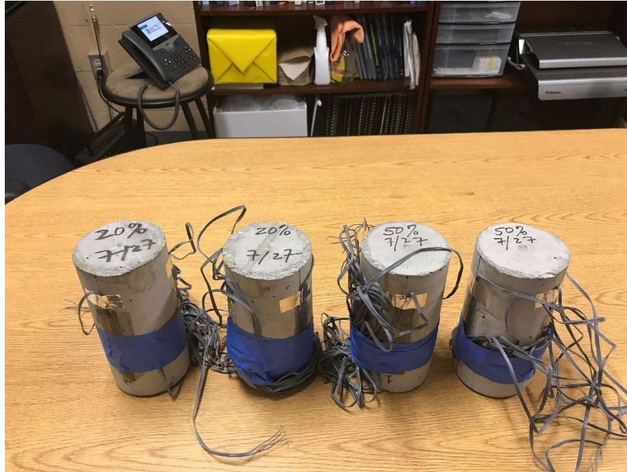
Figure 12.12.57 Specimens Underwent Full Stress-Strain Testing
