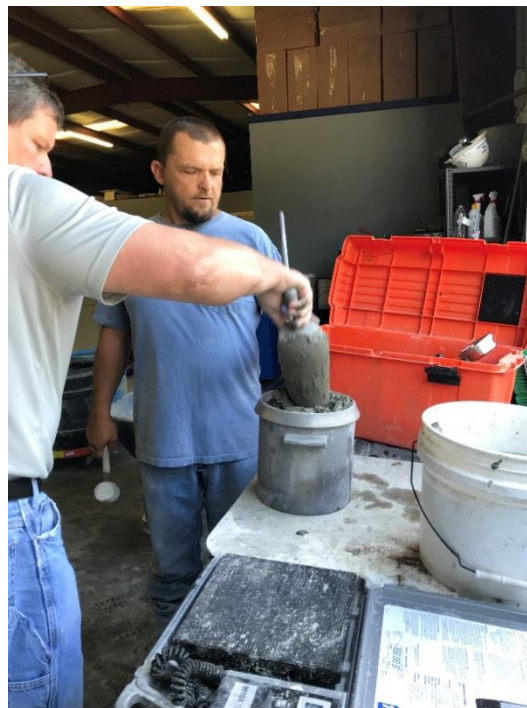
Figure 12.12.50 Fresh Concrete Unit Weight and Air Content Test
