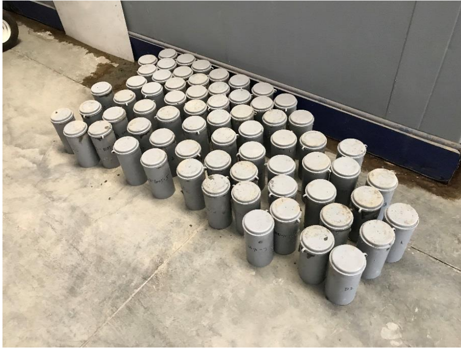
Figure 12.12.51 First 24 Hours Before Demold and Move to Curing Room
