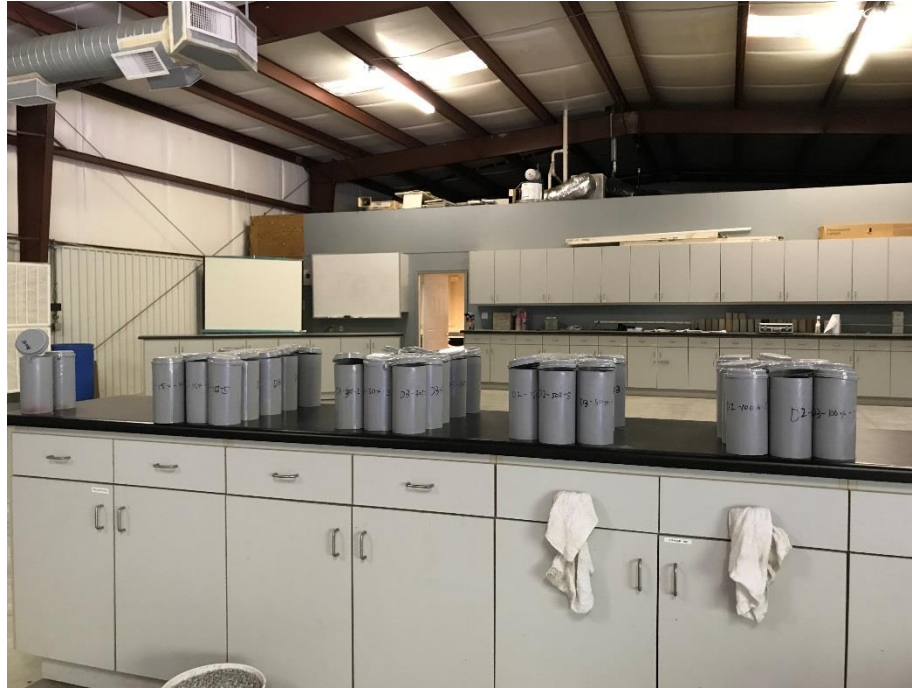
Figure 12.12.41 4” Molds Prepared for Casting Cylinders
