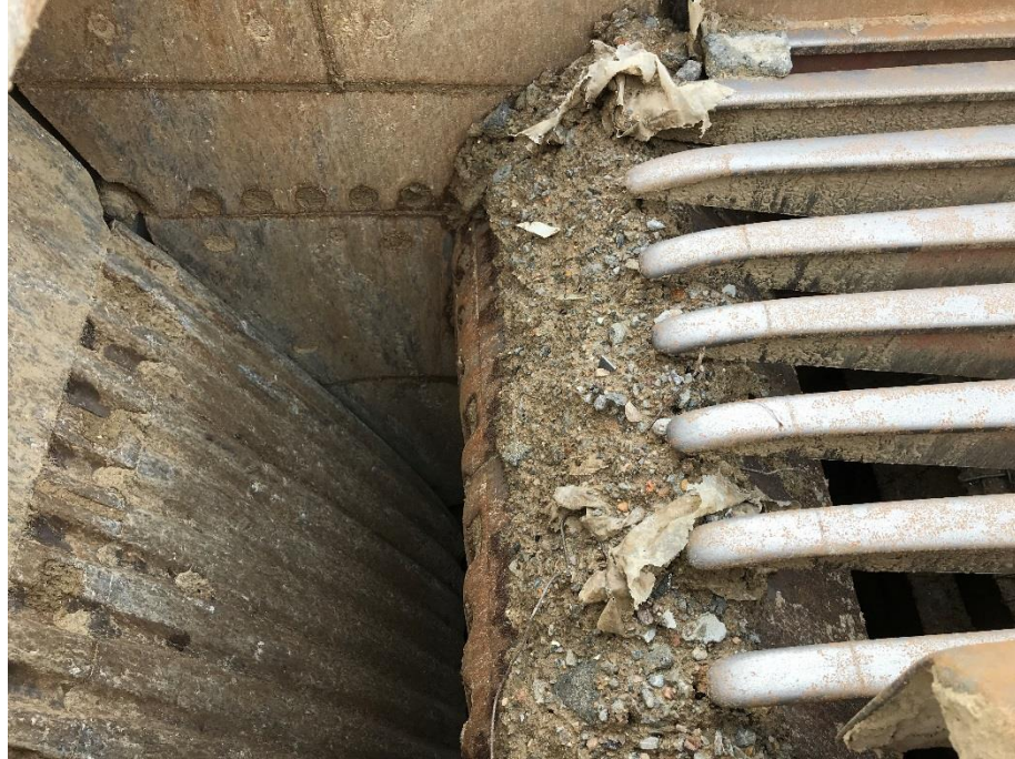
Figure 12.12.9 Jaw Crusher of the Terex Finlay Machine
