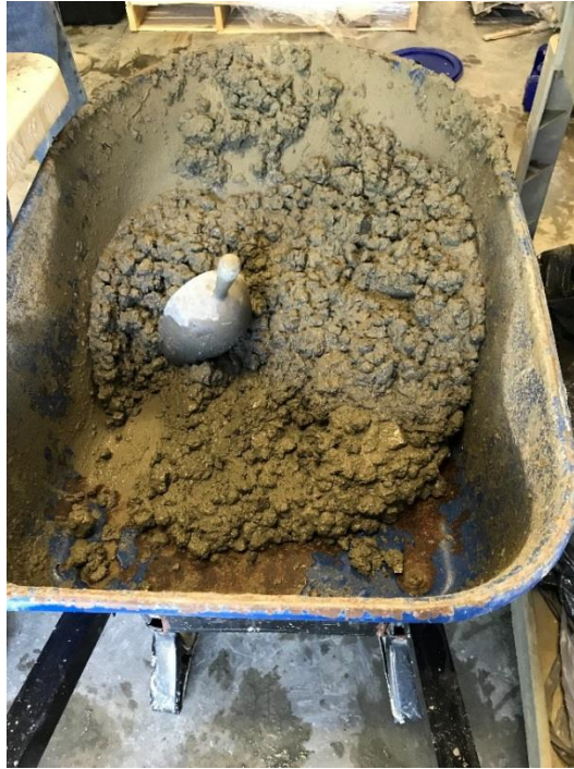
Figure 12.12.45 Fresh RCA Concrete Discharged from Mixer
