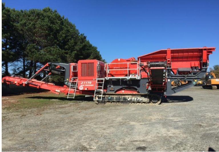
Figure 2.1.2 Terex Finlay J-1170 Compact and Tracked Jaw Crusher
