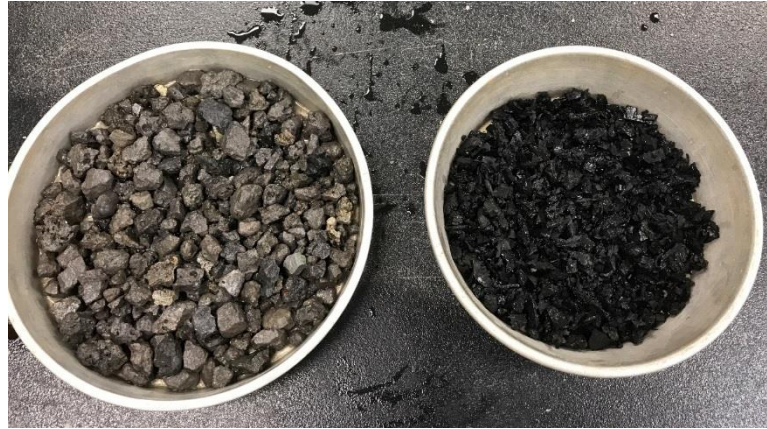
Figure 6.3.1 EAF Slag and Shredded Scrap Tire Rubber (STR) for the Pioneer Study
