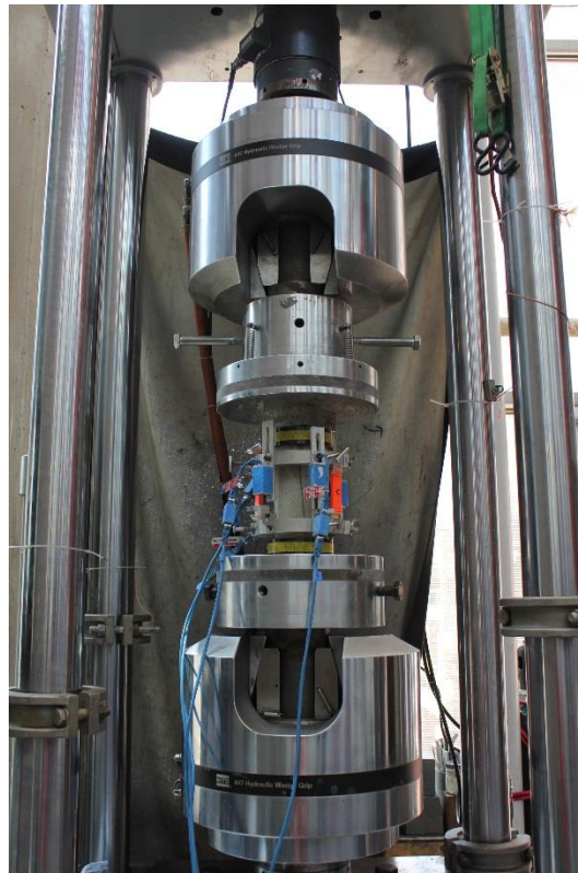
Figure 12.12.58 Repetitive Cyclic Testing to Obtain Full Stress-Strain
