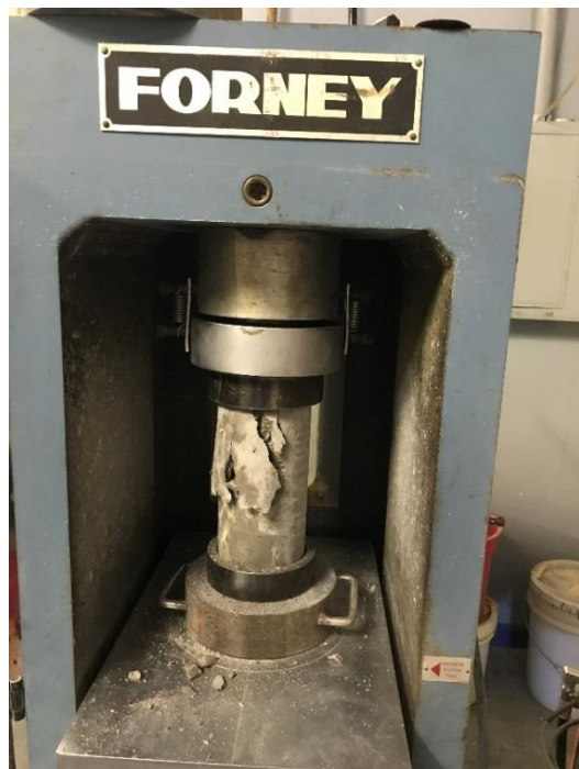
Figure 12.12.54 Breaking Concrete Cylinders
