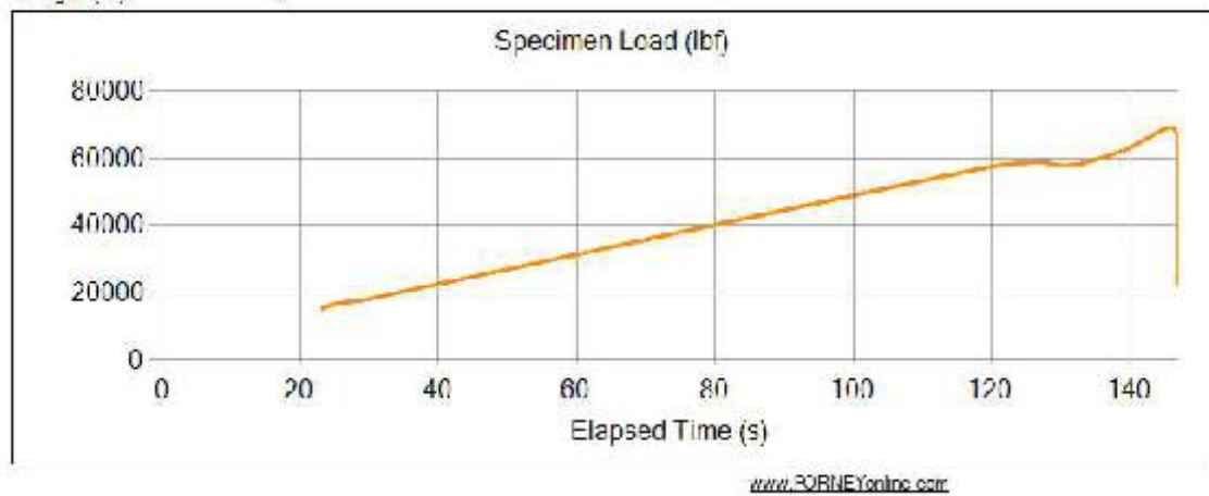
Figure 12.9.71 50%EAF Slag + 50%RCA Concrete 90-day Strength
