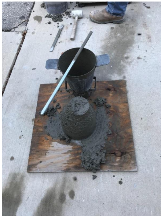
Figure 12.12.48 Slump Test for Fresh Concrete Containing RCA
