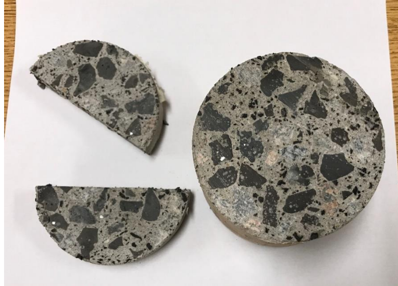
Figure 6.3.3 Concrete Containing Nucor Steel Slag after Pressure Steam Treatment
