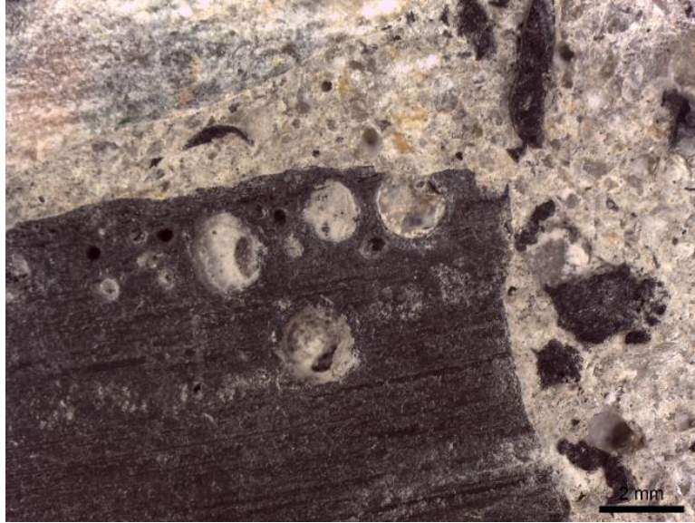
Figure 6.3.6 Pores on the Surface of the Slice, Leica MZ125 LED Lighting 8.0 ×
