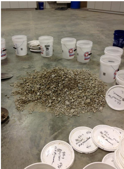
Figure 12.12.26 Coarse Aggregate for the Concreting
