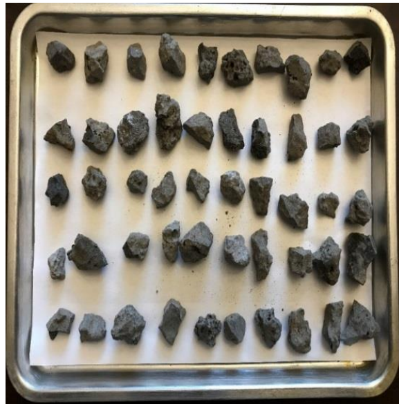
Figure 4.3.4 EAF Steel Slag Aggregate After Pressure Cooker Treatment
