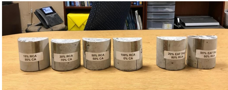
Figure 6.1.1 Saw-Cut Specimens Containing RCA and EAF Slag Coarse Aggregate
