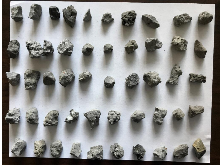
Figure 12.12.35 EAF Slag is Volumetrically Stable After Testing
