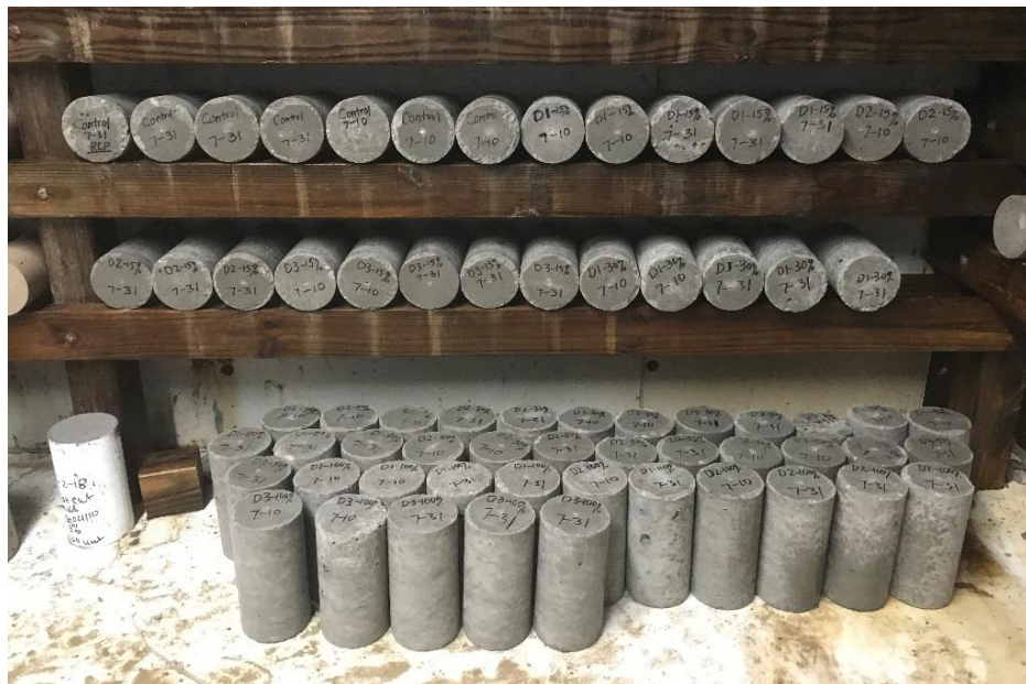
Figure 12.12.52 Cylinders in Curing Room for 7-, 28-, 90-day Tests
