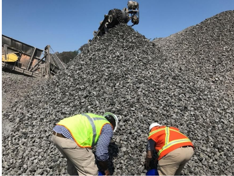
Figure 4.3.3 Sampling of Steel Slag Aggregate at Nucor Steel in Hertford County, NC
