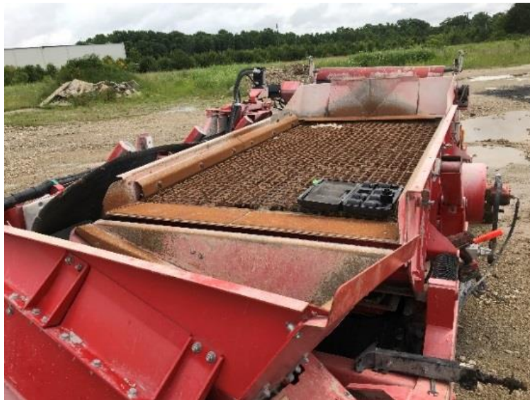
Figure 4.2.6 A Separate 1.5-Inch Screener is Selected and Used for Sizing Crushed RCA
