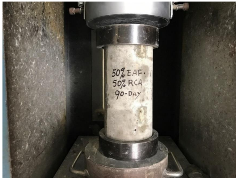
Figure 5.3.3 Breaking 90-day Cylinder Containing RCA and EAF Slag Aggregate
